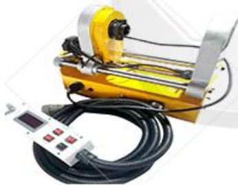
6.Internal hole repair welding machine
